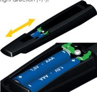
Once the batteries have been inserted, close the battery compartment lid again and the radio transmitter is operational.
